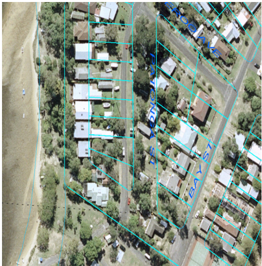
Current landbase parcel locations in blue overlaid on ortho-rectified imagery. This illustration highlights the magnitude of the discrepancy in some parts of the EnergyAustralia supply area.
